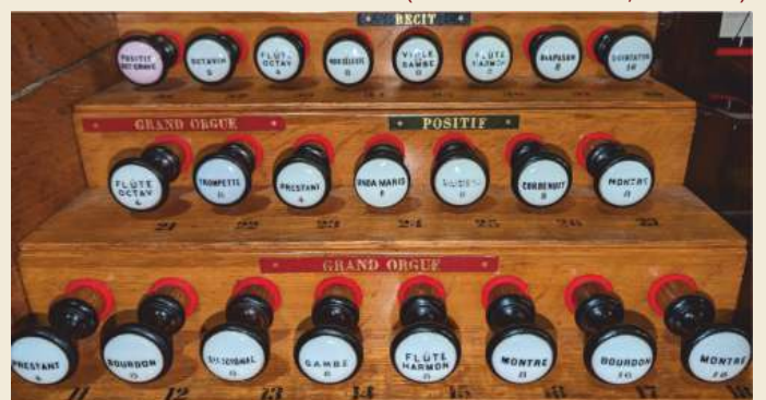
Example of stop knobs as found by the organist at the console (here at Saint-Sernin, Toulouse).
