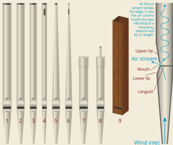
Examples of flue-pipe forms: 1 Flute; 2 Principal; 3 Salicional; 4 Viola da Gamba; 5 Spitzflöte; 6 Gemshorn; 7 Bourdon; 8 Chimney Flute; 9 Wooden Flute pipe.
